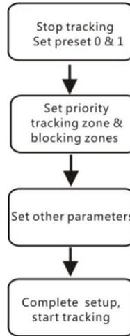
Preset 0 and Preset 1 are set as presets of full view image, or as presets of any zoom or position. When there is no target, camera will return to preset 0 or preset 1. Please refer to Basic Setting.
