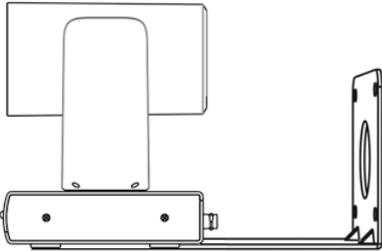
1. According to diameter and position of the 4 installation holes (As shown below) on the bracket, drill 4 holes on the wall and fix the bracket onto the wall by using 4 screws which should be prepared by you.
