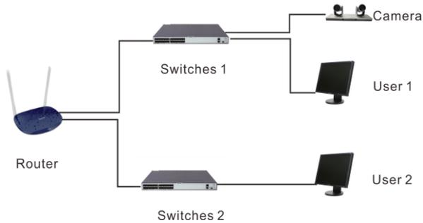
Please refer to the above diagram, user1 and user 2 are in the same router, they are considered as in the same LAN, connect the camera to the same LAN as where the PC is, and refer to below instructions as how to use the application software, then the camera can be found and connected from the online device list.
