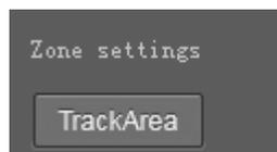
The tracking zone and blocking zones (up, bottom, left and right limits) have to be set. The tracking zone is an area where the targets are.
