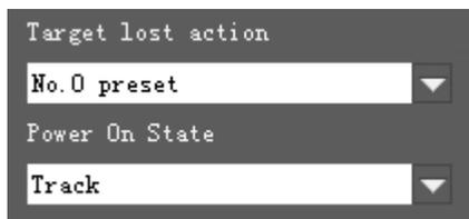
**Target Lost Action:** Used to define the action to be performed if the camera loses the tracked object for a period of time.
