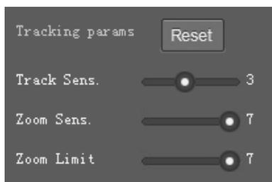
**Tracking Sens:** Set sensitivity of tracking enable to detect and track. High sensitivity easily, and not lose the object.
